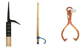
Serving the market for over 100 years and made of high-quality materials, Dixie Industries brand utility accessories, such as pole tongs, pike poles, cant hooks, and peavies, are used throughout the utility industry to move, roll, slide, or float poles into position.
