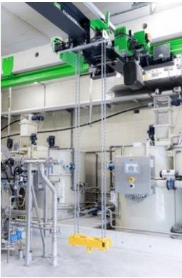
The single-girder suspension crane, realized with the CraneKit from STAHL CraneSystems (Image source: Summer Metalltechnik)
