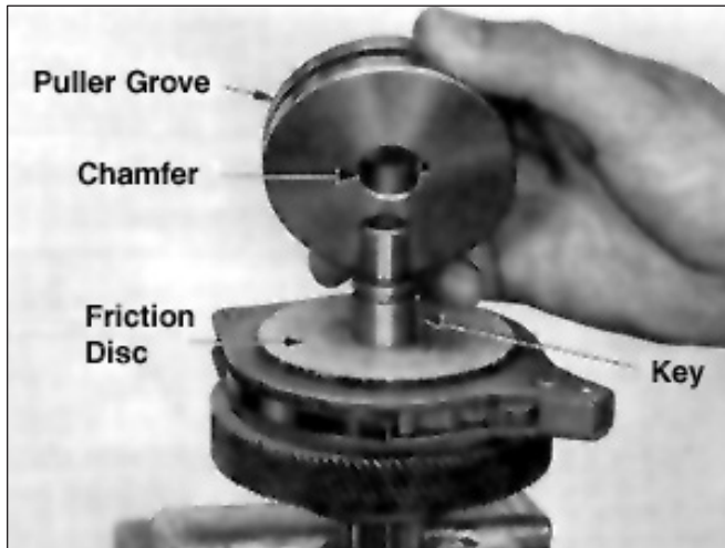
Figure 5-7. View Showing Load Brake Flange Removed
