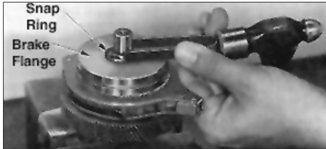
Figure 5-6. Remove Snap Ring From Load Brake Shaft
