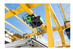
The compact AS 7 wire rope hoist with monorail trolley acts as a powerful auxiliary hoist.
