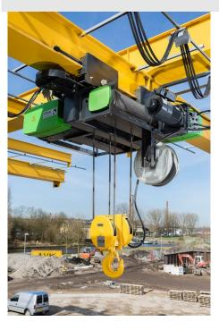
The SH wire rope hoist as TwinDrive concept combines the high FEM 3m classification with hoisting speeds of up to 25 m/min and a very low headroom. The guide roller is positioned horizontally next to the hoist (top left in the photo).
