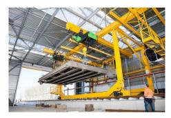
The wire rope hoists can be coupled for tandem operation, for example to lift the partition wall for shortening the flume. Lateral jibs enable loads to be taken up outside the gantry crane.
