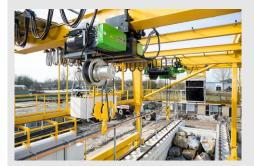
This wire rope hoist has been developed to assist the scientists building the test dykes with its fast, precise lifting movements.
